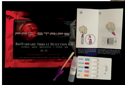
Pro Strips Rapid Screening System, developed by ADVNT Biotechnologies LLC, is the first advanced multi-agent biowarfare detection kit that tests for anthrax, ricin toxin, botulinum toxin, plague, and SEB (staphylococcal enterotoxin B).
