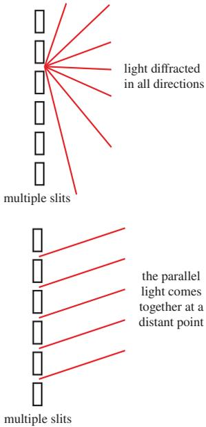
**C.3 Figure 36** Light diffracted at each slit undergoes interference at a distant screen.
