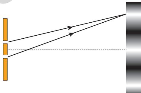
**C.3 Figure 32** Paths taken by the rays from each slit to the first maximum
