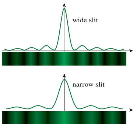
**C.3 Figure 28** Notice that with a narrower slit the pattern is wider but less intense.
