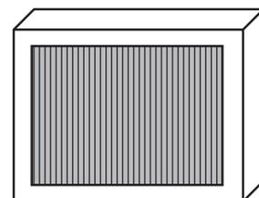
**C.3 Figure 35** Diffraction grating (the number of lines per millimeter can be very high: school versions usually have 600 lines per millimeter).
