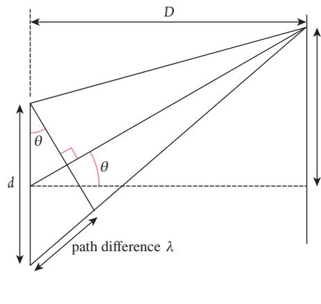
Since this is the first interference maximum, the path difference between the waves must be  $\lambda$ . If we fill in some angles and lengths as in Figure 33 we can use trigonometry to derive an equation for the separation of the fringes.
