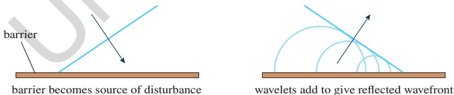
**C.3 Figure 5** Reflection of a plane wavefront.
