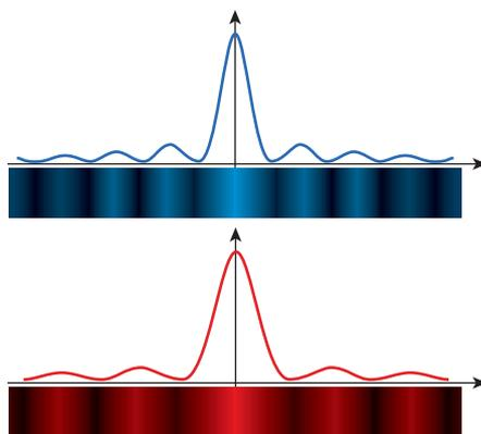
**C.3 Figure 29** Same size slit but different wavelength light; longer wavelength gives a wider pattern.
