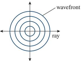
**C.3 Figure 1** A circular wavefront spreading out from a point.
