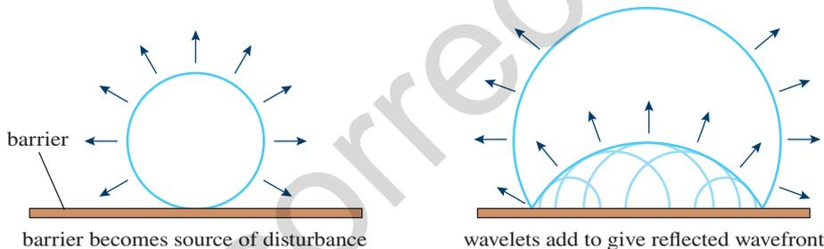
**C.3 Figure 4** Reflection of a circular wavefront.
