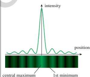
**C.3 Figure 22** Single-slit diffraction.
