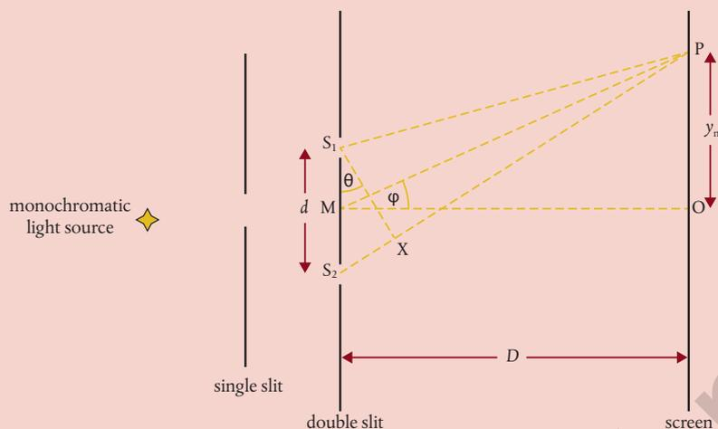
The distance  $S_1S_2$  is  $d$ , the distance between the double slit and screen is  $D$  and  $D \gg d$  such that the angles  $\theta$  and  $\phi$  shown on the diagram are small.  $M$  is the midpoint of  $S_1S_2$  and it is observed that there is a bright fringe at point  $P$  on the screen, a distance  $y_n$  from point  $O$  on the screen. Light from  $S_2$  travels a distance  $S_2X$  further to point  $P$  than light from  $S_1$ .
