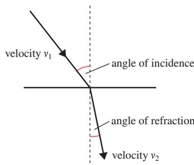
**C.3 Figure 8** Angles of incidence and refraction.
