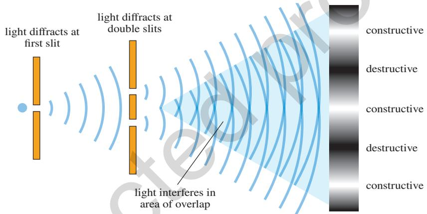
**C.3 Figure 31** Double-slit interference.
