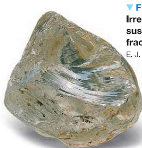
B. Conchoidal fracture (Quartz)
